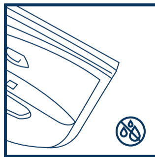
Make sure the surface is completely dry before starting application of Q 2 Purify Coat.
